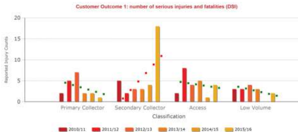
Figure 3: Serious injuries and fatalities (DSI) by ONRC category - Sourced from ONRC performance measures reporting tool
