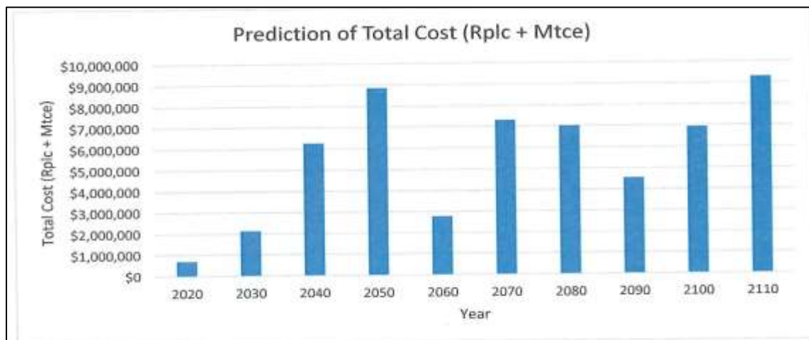
Figure 3-6: Bar chart for predicting retaining wall replacement and maintenance costs for the next 100 years
